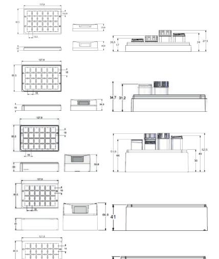
Micronic 24-1 rack dimensions and tube in rack dimensions Left: 1.50ml externally threaded Hybrid tubes with Screw Caps. Right: 3.00ml externally threaded Hybrid tubes with Screw Caps.
