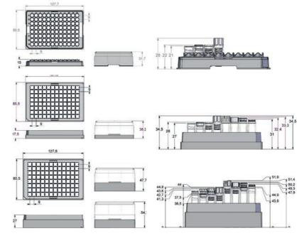
Micronic EFC 96-1 rack RM dimensions and tube in rack dimensions Left: 0.50ml internally threaded tubes with TPE Push Caps / Low Profile Screw Caps or Screw Caps.
