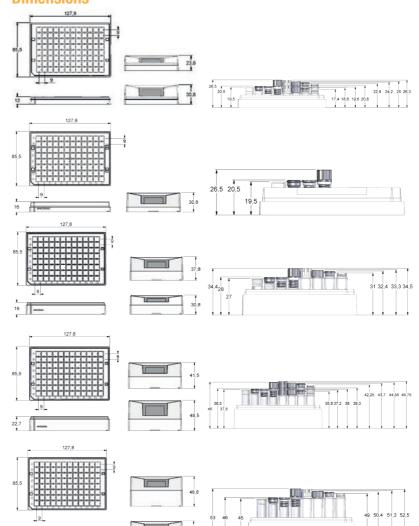
Micronic 96-1 rack dimensions and tube in rack dimensions
